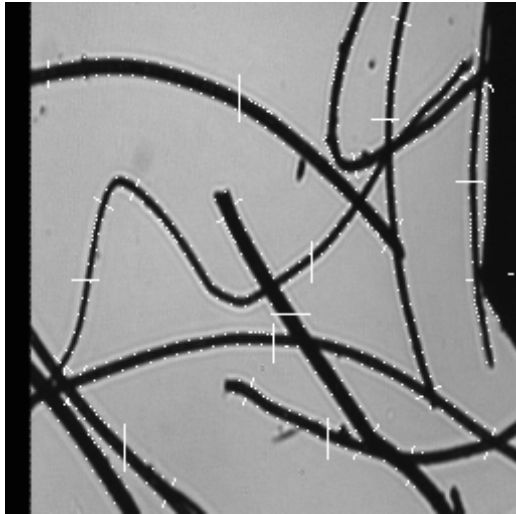
Fig. 1. Hair fibers of ibex ( Capra sibirica ) during analysis by optical fiber diameter analyzer.
